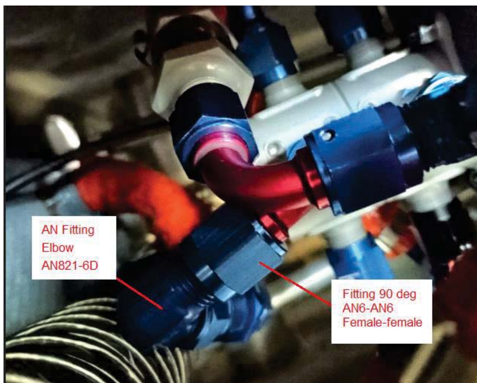
Pic. 3.20 Connect the Engine Supply fuel line upper side view
