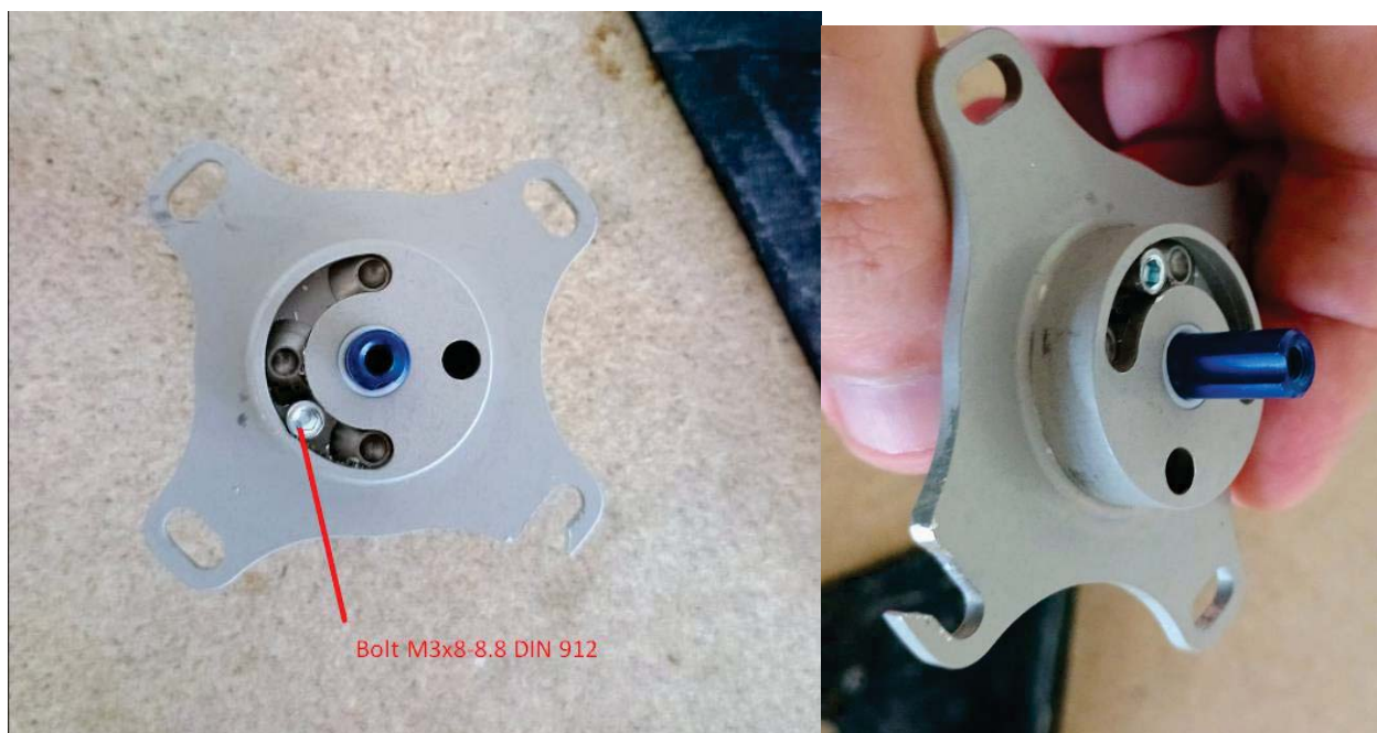
Pic.3.12.1 Adjusting of Fuel selector mounting plate
