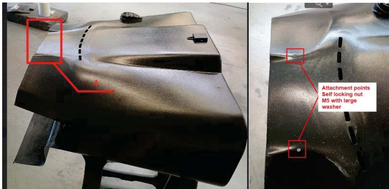
Pic. 3.9.2 Dismount upper attachment points of instrument console
