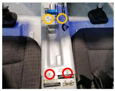
Identify the ball/rod end on the push-pull cable. The ball end is found underneath the throttle box.
