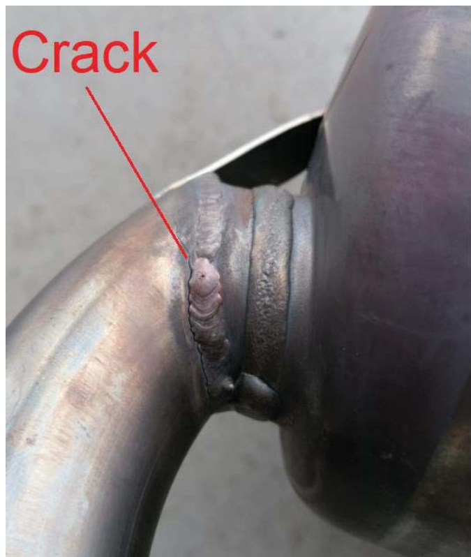
Fig. 3-1 - Exhaust pipe crack (example)
