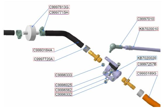
b. Clear straight disc-shaped plastic filter straight in line with the fuel lines. The filter is located directly downstream of the fuel valve.
