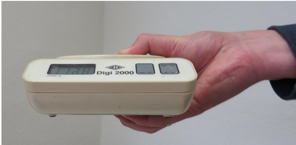
Fig. 4 – “calibrate” hand force to 1.0 .. 1.5 kg force
